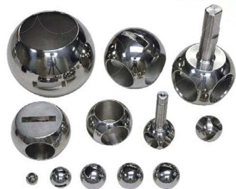
A v-port ball valve has a "v" shaped ball instead of a round-bore ball. This allows the orifice to be opened and closed in a more controlled manner with a closer to linear flow characteristic PVS FLOW CONTROL provides several v-port balls in Series 35 with different angles of "v". Note that the long-term throttling operation in a certain percent open is not recommended. For Cv, please see Flow Coefficients (Cv) of V-port Ball Valve.
